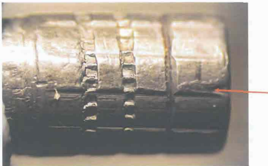
Figure 23. Feature on the base of bullets (arrowed). This is most probably the result of gas erosion.
